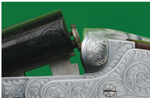
Side clips on this close-up of the 28-gauge side-by-side from Huglu. These clips are a great touch to these somewhat older guns.
